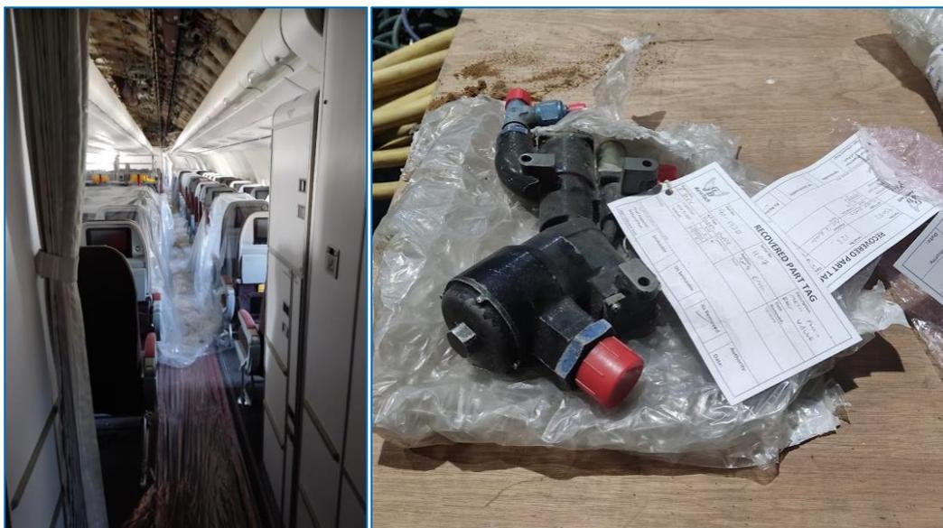
Figure 42. Aircraft cabin during disassembling (left) and recovered part (right). (Envisa, 2022)
