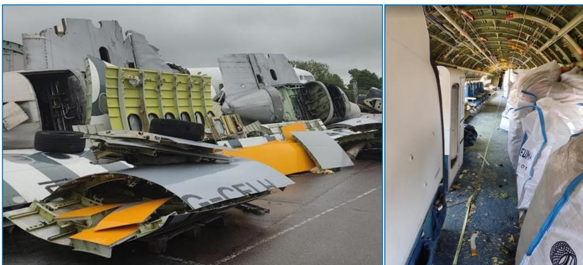
Figure 46. Dismantled aircraft sections (left) and interiors preparation for dismantling (Envisa, 2022)
